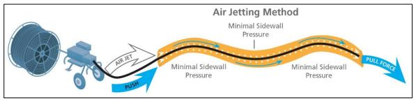
Figure 6: Typical Air-assisted Jetting Method (not to scale)
