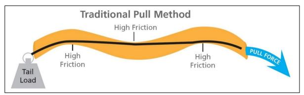
Figure 5: Traditional Pulling Method (not to scale)
